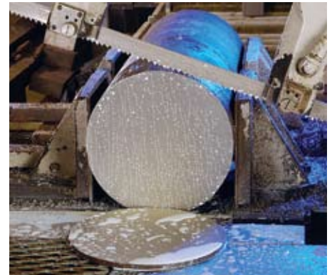
START TO CUT MATERIAL AT REDUCED CUTTING RATE
