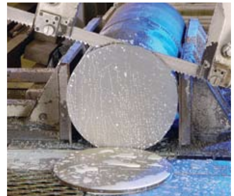
AFTER BREAK-IN WHEN THE BLADE HAS FULLY ENTERED THE WORK-PIECE, INCREASE THE FEED RATE OVER A SERIES OF CUTS UNTIL THE RECOMMENDED CUTTING RATE IS ACHIEVED
